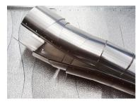
Automatic rounding and beading of Bend segments, Isometric bends, T-piece and Fitting pieces.
